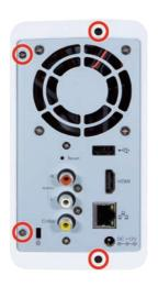
2. Use a Philips screw driver to release the screws.
