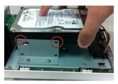
13. Secure the HDD with the screws provided in the accessory box with a Philips screw driver. There are four for each HDD; two for each side of the tray.
