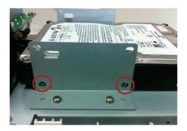
9. Secure the HDD with the screws provided in the accessory box with a Philips screw driver. There are four for each HDD; two for each side of the tray.
