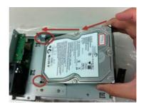
6. Once the HDD is placed into the tray, you should see a gap between the HDD and the SATA connector.
