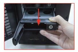
3. Place the HDD in the tray and the bottom of the tray.
