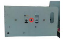
4. Insert the HDD to HDD tray. Please push the HDD until the SATA connect is connected properly, and lock the HDD Screw on left and right side.
