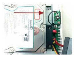
8. Make sure the screw holes on the HDD are aligned with the ones on the tray.
