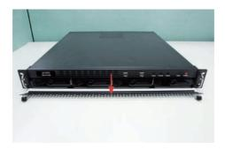
4. Remove the HDD tray by pulling the latch.
