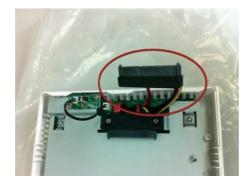
11. Make sure the HDD is securely attached.
