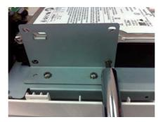
10. Install the top HDD by attaching it to the corresponding SATA cable first.
