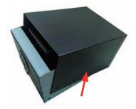
3. Removing the screws on the HDD Tray left and right side.
