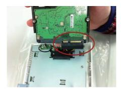
12. Place the HDD to the tray and make sure the screw holes on the HDD are aligned with the ones on the tray.
