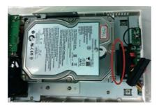
7. Attach the HDD to the SATA connector by sliding it towards the connector.
