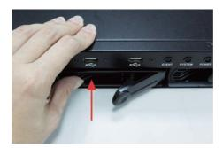
9. Secure the tray by pushing in the latch, which locks the tray with the unit.
