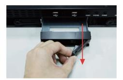
6. Once the tray is removed from the unit, notice there are four holes, which are used to secure the HDD.
