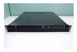
2. To remove the front plate, turn the tool-less screws on both sides counter-clock wise to loose it from the unit. Please note the screws will still be attached to the front plate even after the screws are completely loosened from the unit.
